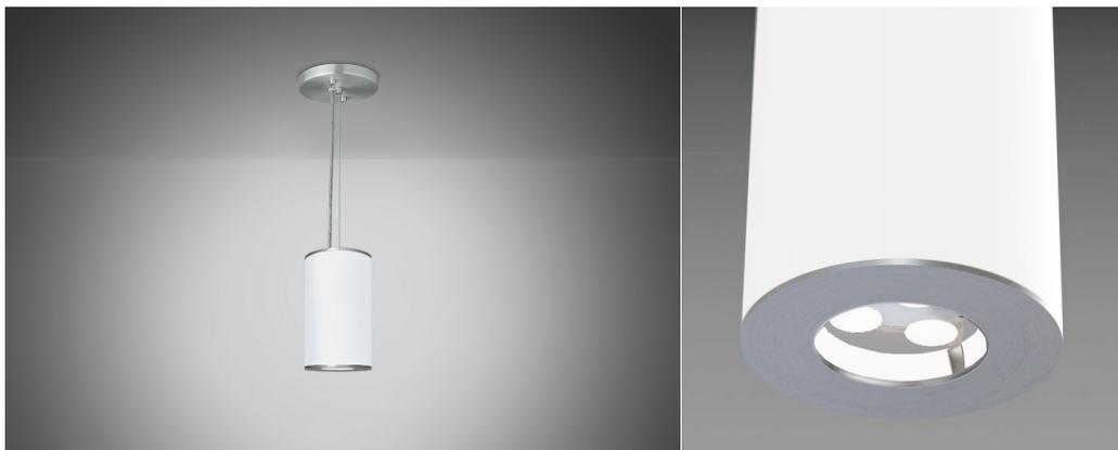
*The VASO utilizes the latest in LED downlight tech, with (3) Mid-power LEDs mounted to a central board with high-efficiency acrylic lensing. Available in narrow, medium and wide beam spreads, the downlight at 12W delivers over 1500 Lumens in the beam.
